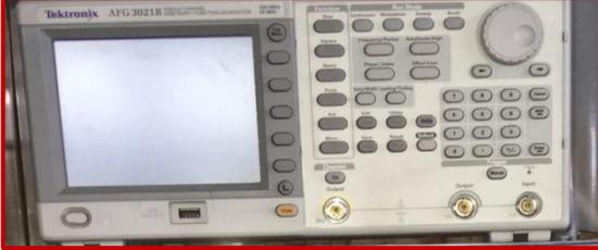
A photograph of the Tektronix AFG 3021B Arbitrary Function Generator. It is a rack-mountable device with a color LCD screen on the left and a control panel with numerous buttons and a large rotary knob on the right. The model number '3021B' is visible on the top left of the front panel.                  |
